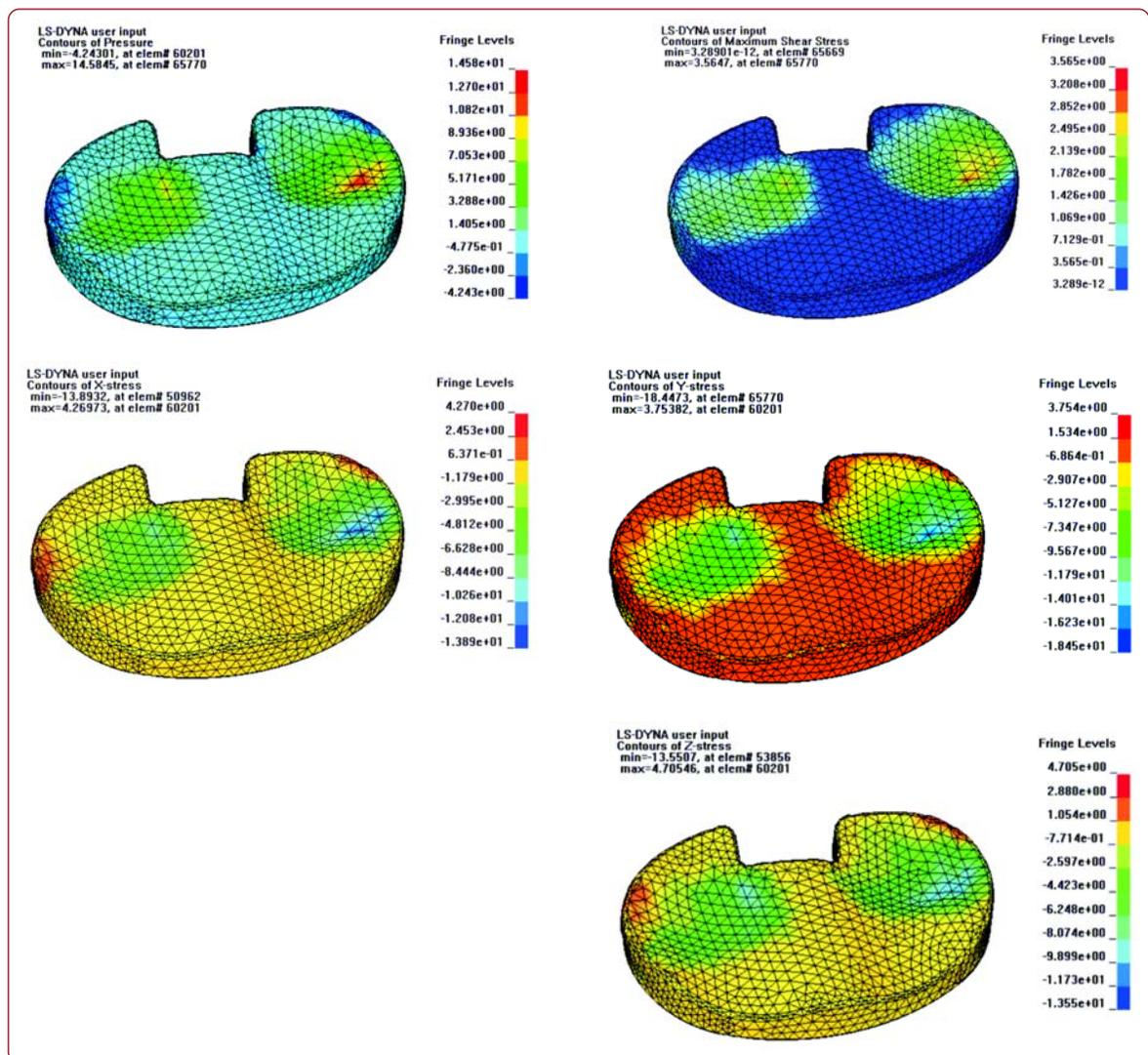
FIGURE 6. Polyethylene contact stress according to finite elements method
