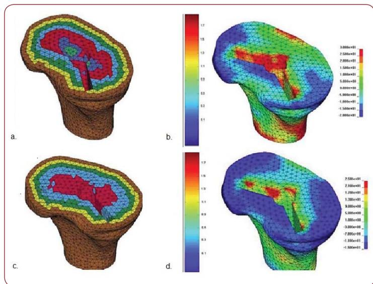
**FIGURE 1.** The distribution of the bone density and the stress concentrations at the level of the bone-prosthesis interface and of the prosthesis proximal tibial extremity, immediately after arthroplasty (a, b) and after 10 months of bone remodelling (c,d).
