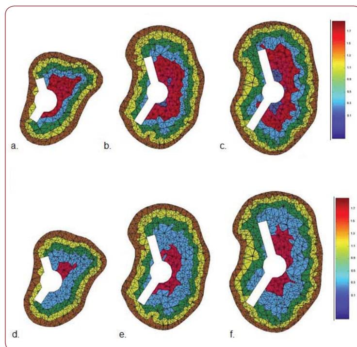
**FIGURE 2.** Series of sections of the prosthesis tibial epiphysis, with bone density distribution before (a,b,c) and after 1- months of bone remodelling (d,e,f).
